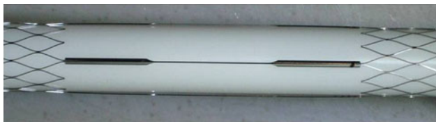
Fig. 1 Tensile test sample incorporated into stent framework
